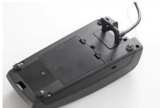
Figure 1: Cable Placed in iPP300 Port
